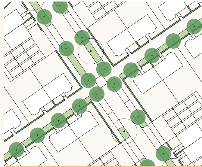
Carriageway narrowing to reduce traffic speeds
