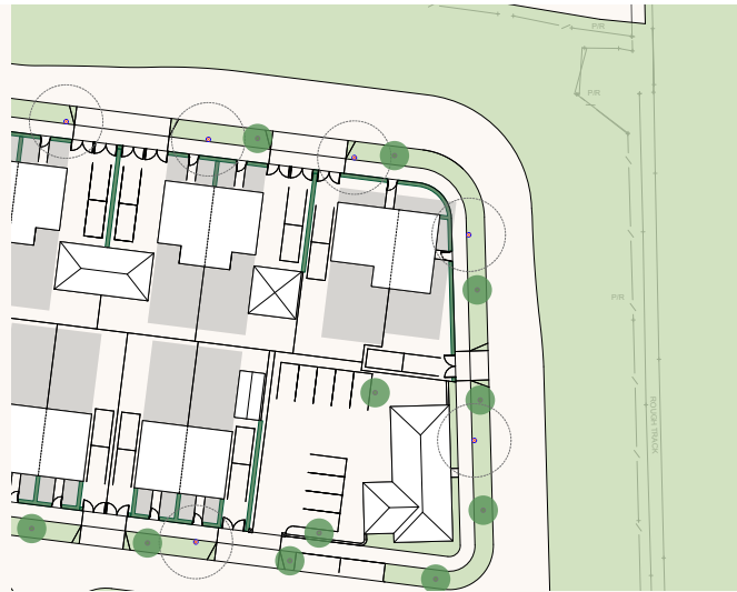
Road alignment with reduced forward visibility that will promote slower vehicle speeds
