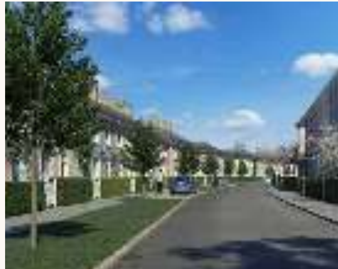
Houses create reduced forward visibility and speed reduction bend
